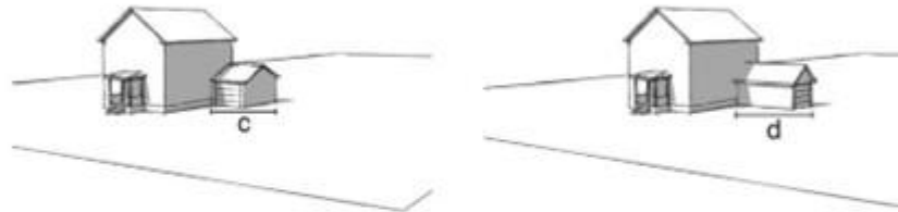
Acceptable location for garage: attached to dwelling; garage is set back behind the front plane of the dwelling at least 1/3 of the depth of the dwelling (c, d).
